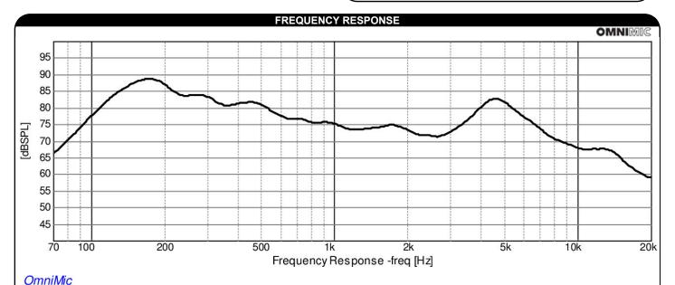
1/3<sup>rd</sup> octave smoothing - measurement taken with transducer adhered off-center on a 12" x 12" x ½" foam core board in an infinite baffle setup.
