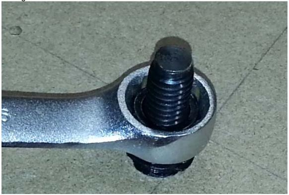
**6.** Once the insert is flush with the speaker cabinet, loosen and remove the nut and spike. The insert will stay in place with most cabinet materials. If the insert begins to back out with the nut, it may be necessary to use a set of pliers to hold the insert in place from the inside of the cabinet while removing the nut.
