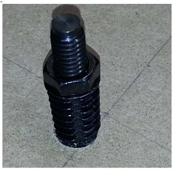
**5.** Use the appropriate wrench to screw the barbed insert into the cabinet by turning it clockwise.
