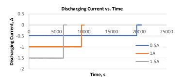
Note: A higher current takes lesser time to fully charge and discharge. 5V input voltage takes the longest time for the battery to be fully charged compared to other input voltage with the same charge current. Charge current is approximately the same when input is higher than 9V, hence, time to fully charge will be almost the same.
