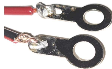
Wires soldered to terminals
