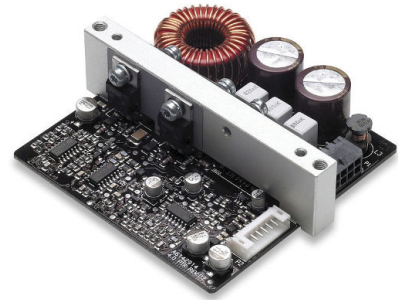
Figure 1: ICEpower500A Size: 9 x 9 x 2.7cm
