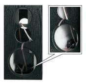
6. Apply some glue to the tube and install it into the tube hole.
